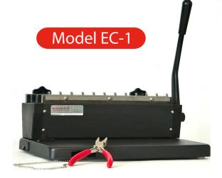
Binding machine with UNIVERSAL PUNCH® perforation system for 20 types of binding (for pitches 3:1, 2:1, 4:1, .2475", 5:1, 2.5:1, 6mm), for double wire loop, plastic coil, Velobind® strips, metal coil, 11- ring Universal Plastic Comb®, 3-ring binders, two ring binders, etc.
